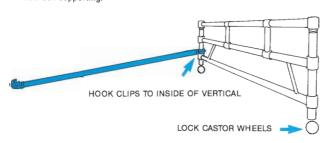
Attach spare end of brace to end of other BASE FRAME. Attach 2nd HORIZONTAL BRACE (yellow hooks) to other side of frame. Attach PLAN BRACE(S) (black hooks) diagonally onto the vertical tube below the lowest base frame rung, or as low down as possible.
