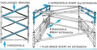
GUARD RAIL EXTENSION: Fit the four PLAIN PLATFORMS first, then the WALK-THROUGH PLATFORM with the hinges of the trap-door to the outside of the tower. Insert the GUARD RAILS, spigots first, into the top of the last frame and secure the interlock clips. Attach two HORIZONTAL BRACES (Yellow Hooks) to the top rung of the GUARD RAIL FRAME and two DIAGONAL BRACES, for rigidity, as shown.
