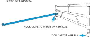
Attach spare end of brace to end of other BASE FRAME. Attach 2nd HORIZONTAL BRACE (yellow hooks) to other side of frame. Attach PLAN BRACE(S) (black hooks) diagonally onto the vertical tube below the lowest base frame rung, or as low down as possible.
