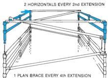
GUARD RAIL EXTENSION: Fit the three PLAIN PLATFORMS first, then the WALKTHROUGH PLATFORM with the hinges of the trap-door to the outside of the tower. Insert the QUARD RAILS, spigots first, into the top of the last frame and secure the interlock clips. Attach two HORIZONTAL BRACES (Yellow Hooks) to the top rung of the GUARD RAIL FRAME and two DIAGONAL BRACES, for rigidity, as shown.
