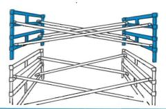
Fit the PLAIN PLATFORMS first, then the WALKTHROUGH PLATFORM with the hinges of trapdoor to the outside of tower.
