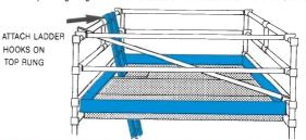
LADDER 'CHANGE-OVER' PLATFORMS: One WALK-THROUGH PLATFORM is required to enable safe ladder change-over on towers with more than one ladder.
