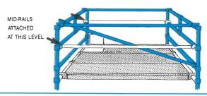
To complete the WORK PLATFORM, first fit the TOEBOARD to allow the trap-door on the platform to open freely. Finally attach the LADDER through the ACCESS PLATFORM, as shown, and clip on stand-off hooks, at base of ladder, to the corresponding rung on the frame. Ensure the access door movement is not impaired.
