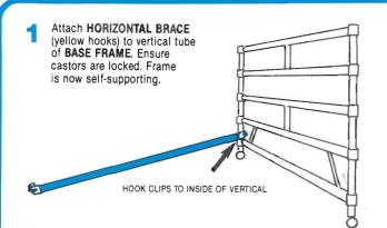
Attach spare end of brace to end of other BASE FRAME. Attach 2nd HORIZONTAL BRACE (yellow hooks) to other side of frame. Attach PLAN BRACE(S) (black hooks) diagonally onto the vertical tube below the lowest base frame rung, or as low down as possible.
